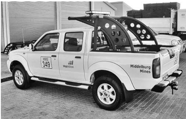
Figure 8: (Above and Below left)The "SWAN" ROPS fitted to utility type vehicles to provide occupant compartment protection a rollover
