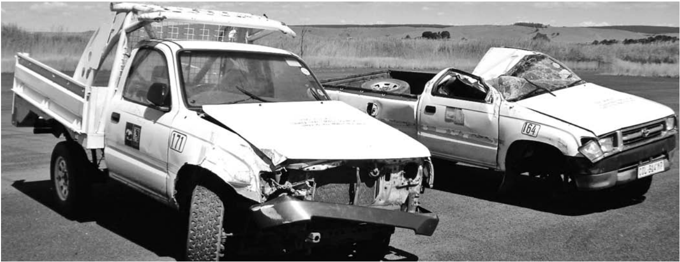
Figure 10: Side-by-side comparison of testing conducted at 60km/h on OEM vehicle with ROPS (left) and without ROPS (right)
