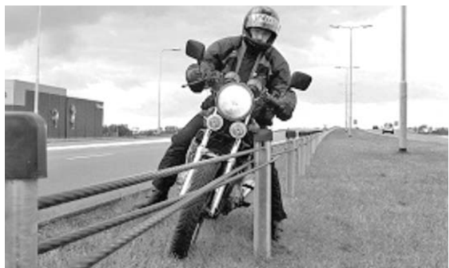
Figure 16: Motorcycle interaction with a typical wire rope barrier. Other interactions involve the motorcyclist sliding or vaulting into the barrier
