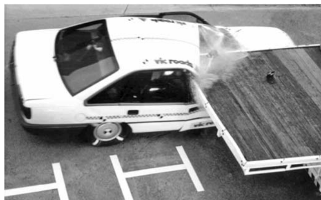
Figure 6: Rear underrun crash test of commodore sedan at 50km/h into rear of tray truck without an underrun barrier)
