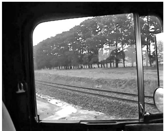
Figure 5: Trawalla level crossing - reconstruction showing the view from the driver's seat and the severely restricted length of track able to be seen. This is an example of very poor visual interface design at the crossing, arising from the level crossing design and the prime-mover cabin design.
