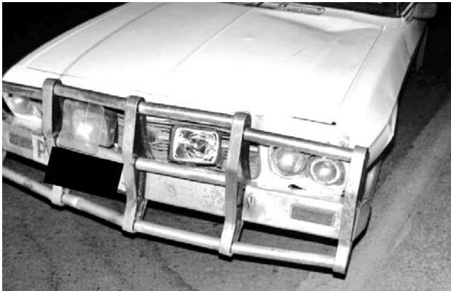
Figure 12: View of a vehicle that impacted a pedestrian [fatality]. Note stiff bull bar structure
