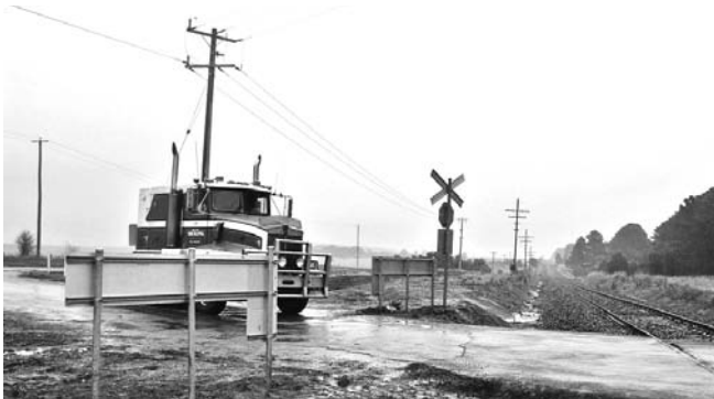
Figure 3: View of the Trawalla level crossing showing a prime mover stopped at the crossing (part of the DVE incident investigation and reconstruction). Note the acute angle of the crossing to the roadway.
