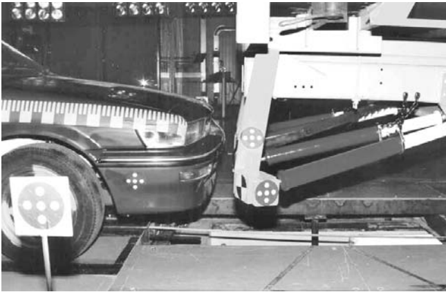
Figure 7 Detail showing interface height of front of Corolla and the underrun barrier.
