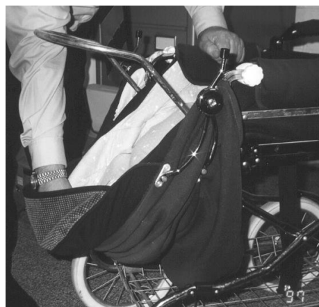
Fig. 1. Emmaljunga pram with backrest off frame and dropped down. Note inverted sleeve forming pocket.
