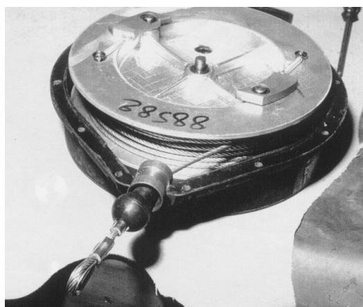
Fig. 10. Inertia reel Fall-arrest device showing the 4mm steel cable.
