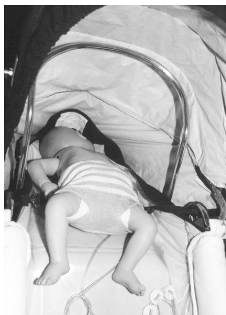
Fig. 2. Emmaljunga pram with backrest off support frame and the head of the baby 'dummy' slid down into the pocket.
