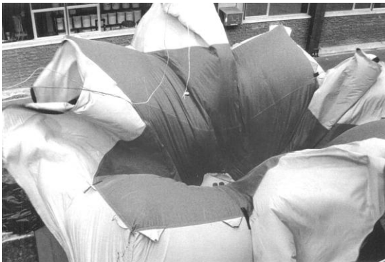
Fig. 6, Centre drop test, double chamber airbag.
