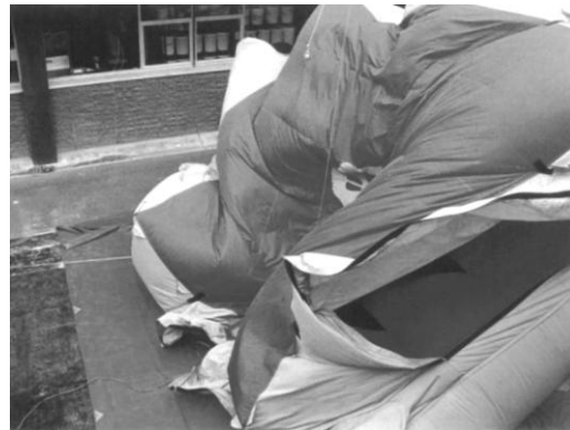
Fig. 7, Edge drop test, double chamber airbag
