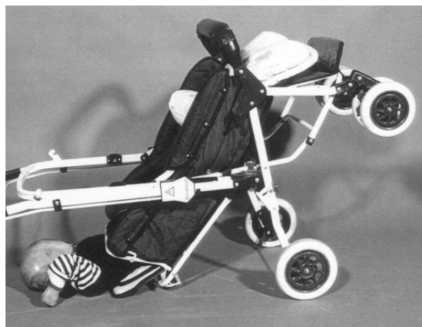
Fig. 4. Unit tipped rearwards, with 'baby' trapped by scissor action of frame.
