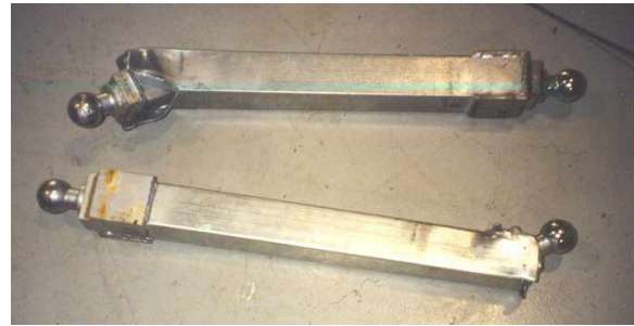
Figure 10. Compression failure of tubes due to overload (wall thickness too low).
